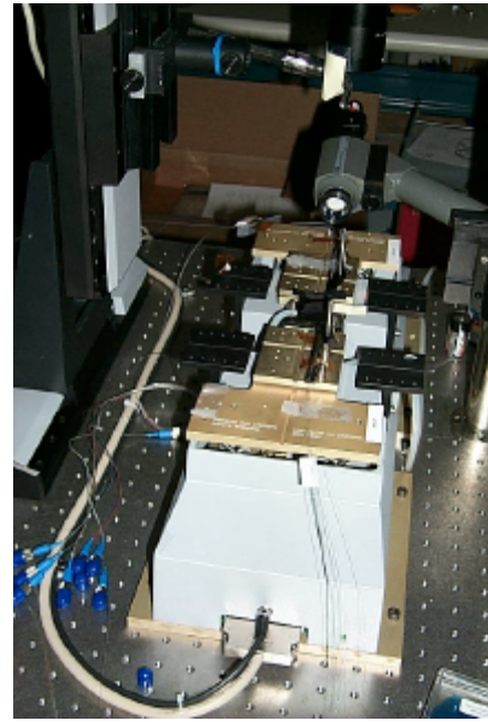
Figure 3. The AWG alignment setup. An IR imager with CCD was used to find first-light. The I/O fiber arrays were each mounted on their own F-206. A PI vacuum chuck for the waveguide was mounted on one F-206's stationary front bracket; the other F-206's bracket was removed; this made for an especially compact assembly. One F-206 controller was used with an XZ assembly of M-500 stages to position a CCD camera above the assembly to facilitate visual alignments.
