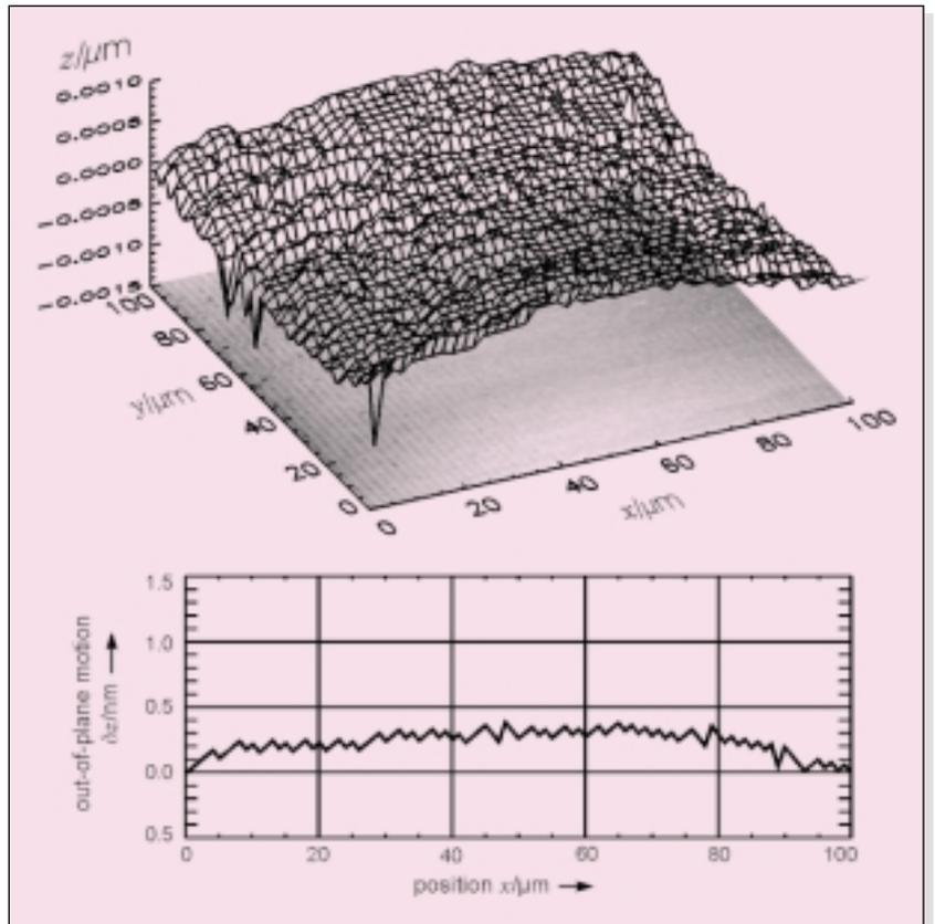
from multiple sensor inputs as well as the individual PZT actuator drive signals. The digitised sensor signals are filtered and linearised with a 4th order polynomial correction. The nominal range of XY and  $\varphi_z$  is  $200 \times 200 \mu\text{m}^2$  and  $\pm 500 \mu\text{rad}$ , respectively. Figure 6 and Figure 7 show the resulting Angstrom-scale out-of-plane motion throughout an XY scan.
