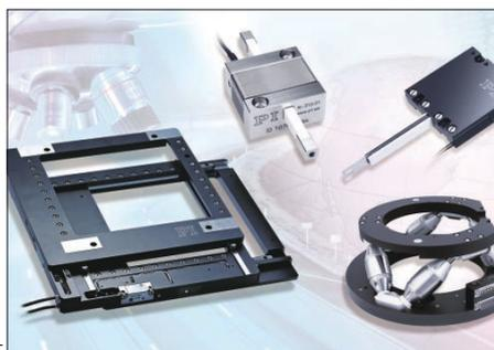
**Fig 3 (left): Hybrid nanopositioning stage design combines properties of piezo ceramic drives and ballscrew drives. Fig. 4 (right): Vacuum compatible, non-magnetic piezo motor actuators and higher levels of integration: XY motor stage and six degrees of freedom hexapod alignment system.**
