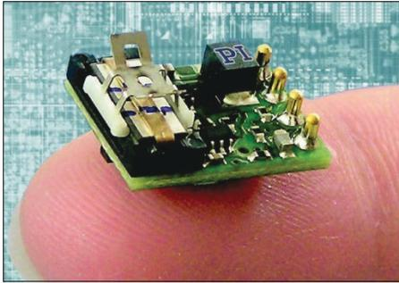
**Fig 5: This shows an example of a miniaturized PCB-mounted piezo motor linear slide for applications such as alignment of micro-optics or autofocus/zoom lenses in mobile-phone cameras.**
