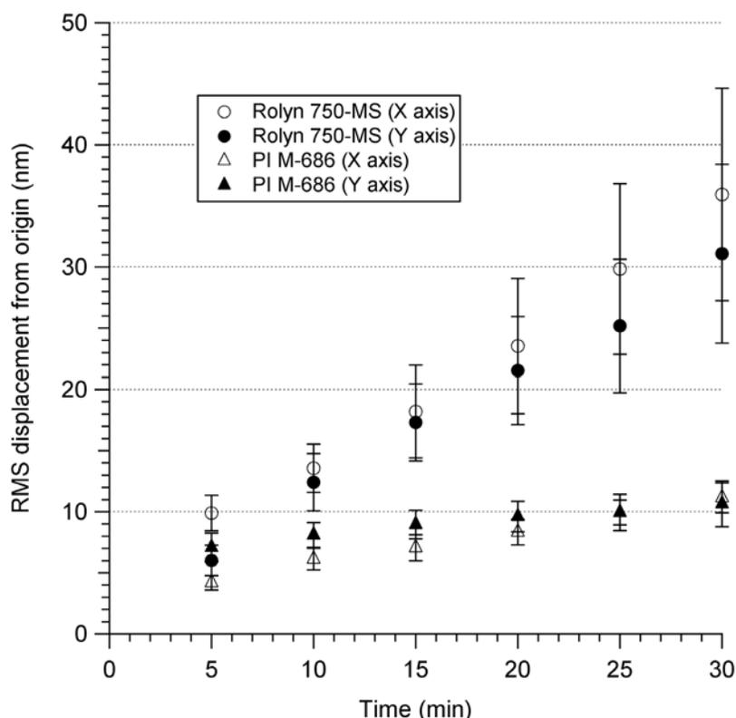
**Fig. (6).** Drift performance of simple screw-driven microscopy stage versus self-clamping piezomotor stage.
