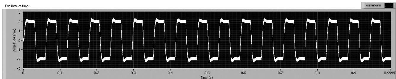
**Fig. (4).** Model position response of nanopositioner in typical point-to-point actuation. Position-vs-time metrology of a model nanopositioner. A 2nm amplitude, 17Hz square-wave actuation is simulated here.
