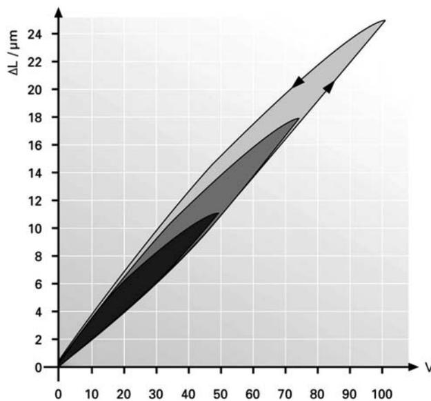
**Fig. (1).** Typical move-dependent hysteresis and non-linearity of open-loop piezo actuation.
