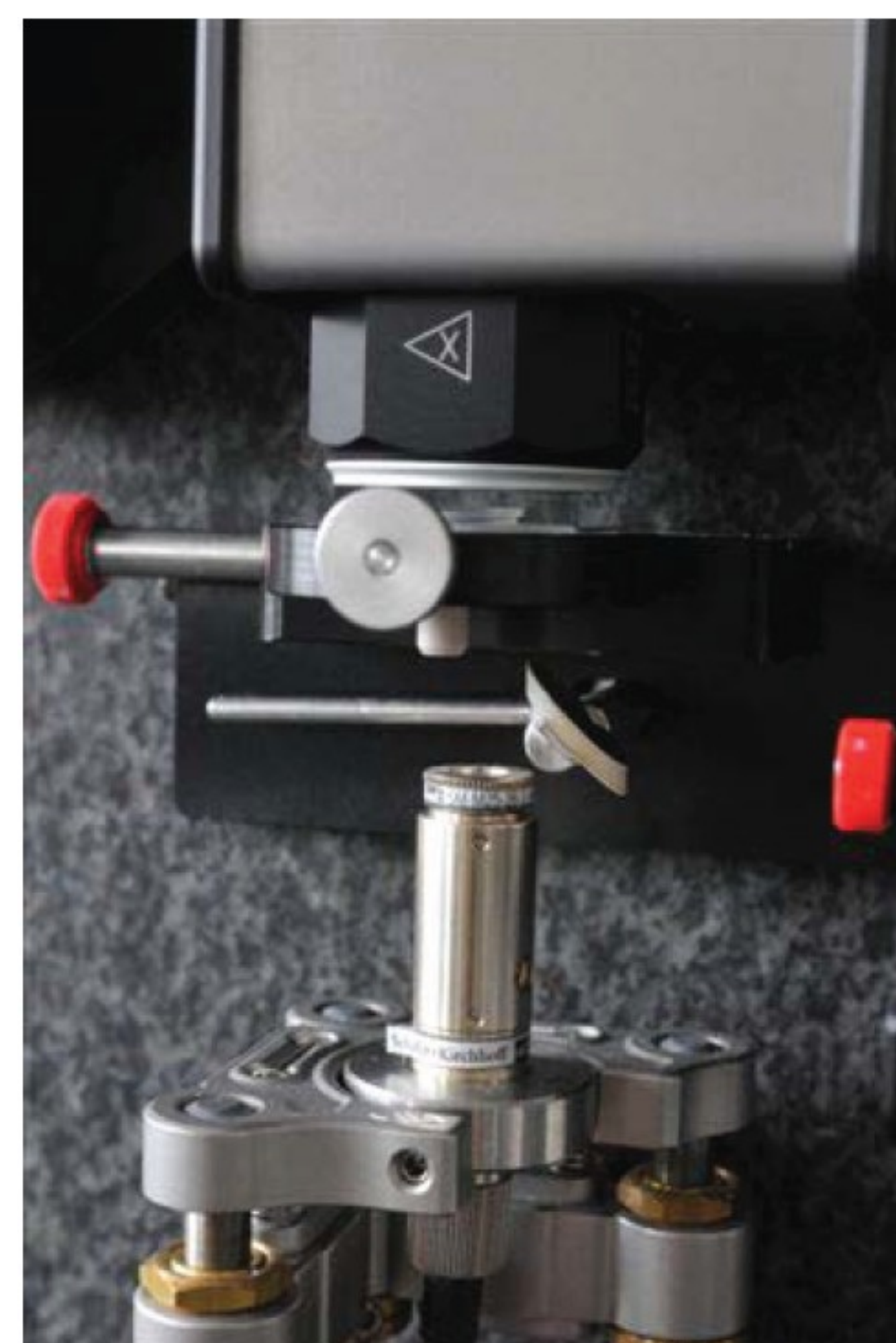
Figure 6. The design of the AFS. The AFS is similar to the Atomic Force Microscope in its basic design, however, the AFS is optimized for force-spectroscopy of short recombinant-proteins. The AFS is fully automatic and operator independent. This is made possible by a set of computer controlled piezo-motors that keep the force-sensor apparatus aligned at all times. Most importantly, a set of piezo-motors constantly optimize the distance between the force-sensing cantilever and the protein layer which is deposited on the surface of a high resolution piezoelectric actuator based upon the PI P-313.00 design.
