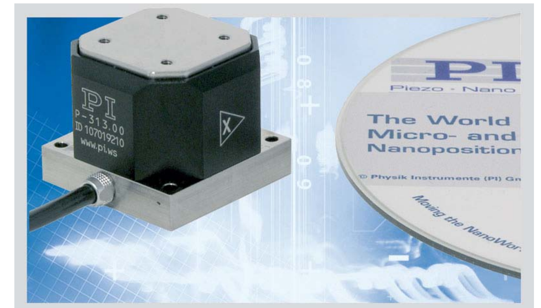
Figure 4. The newly designed P-313.00 piezoelectric actuator from Physik Instrumente. At the heart of this instrument is the integrated XYZ piezo positioner with its new drive principle: A monolithic assembly of three stacked elements of the linear material (with the X and Y elements operating in shear mode and the Z element actuating longitudinally) provides 1x1x0.8 micrometer travel with resolution surpassing 20 picometers. Since the novel piezoelectric material exhibits sub-nanometer hysteresis and a highly monotonic voltage-displacement relationship, no position sensor or servocontroller is needed. Though the 4kHz resonant frequency in X and Y and 11kHz in Z is higher than previous mechanisms, the most significant positioning bandwidth improvement comes from elimination of the sensors and servo loop that would otherwise be necessary. Following-error is thus largely eliminated compared to earlier devices. The resulting combination of sub-nm hysteresis, sub-nm nonlinearity and improved tracking fidelity yields highly repeatable single protein force spectroscopy measurements.
