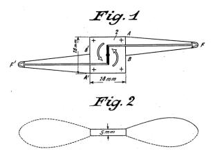
**Figure 1.** Piezoelectric oscillating element to obtain mechanical movement as described in the US Patent invented by Meissner [1].
