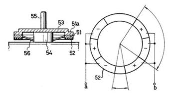
Figure 11. First commercialized ultrasonic motor proposed by Sashida [35].
