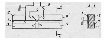
Figure 8. Bidirectional piezoelectric motor designed by Bansiavichus [7].
