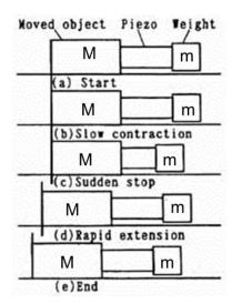
Figure 15. Operating principal of impact-drive proposed by Higuchi in 1986 [53].
