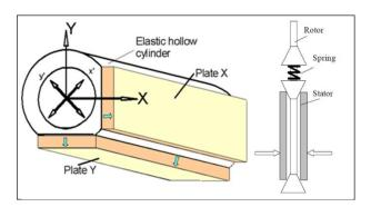
Figure 10. Metal tube piezoelectric ultrasonic motor [34].
