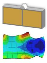
**Figure 6.** Single-mode excitation type ultrasonic motor from Physik Instrumente (PI). The excited single mode of the stator makes the pushing point to have an oblique impact to a sliding element [22].
