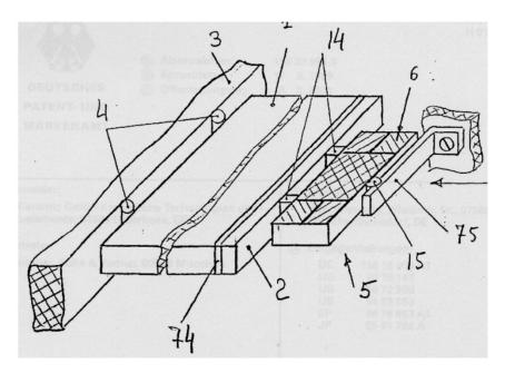
Figure 12. Two-phase motor from Physik Instrumente (PI) [39].
