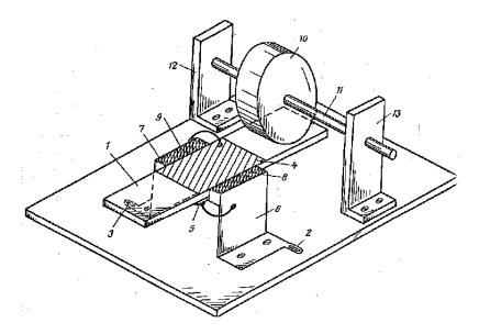
Figure 3. Piezoelectric motor introduced by V. Lavrinenko in 1965 [3].
