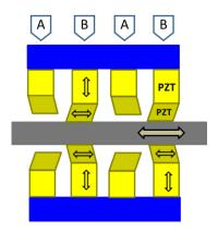
Figure 17. Piezo-walk drive motor at PI [24].
