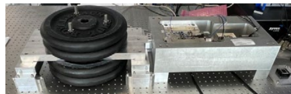
Figure 1: Single-axis piezo AVC test setup.
