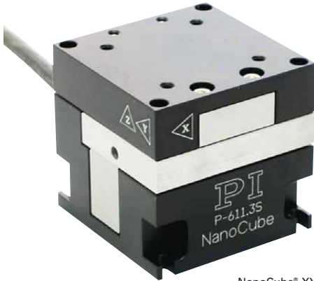
NanoCube® XYZ-nanopositioning system, 100 x 100 x 100 µm closed-loop travel range, resolution 1 nm
