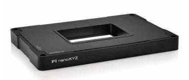
The low profile of 20 mm and special design to allow for a full slide to be mounted at the bottom set Plnano™ piezo microscope stages apart. The Plnano™ Trak version shown above is optimized for extremely fast motion and provides sub-nanometer resolution in up to three axes
