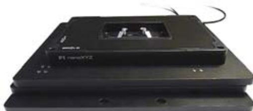
PInano™ XYZ piezo scanner mounted on a M-545K Microscope stage. The XYZ piezo nanopositioning stage provides <1 nm resolution and 200x200x200μm scanning range. The high stability and autolocking feature of M-545 provides significant advantages over other microscope stage designs when using fast piezo scanning stages.
