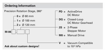
with zero-backlash gearhead and shaft-mounted encoders (2048 counts/rev.). The gear ratio of 29.6:1, provides higher resolution than the direct drive motors.
