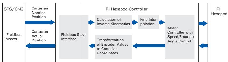
The Hexapod controller acts like an intelligent drive. Due to the exchangeability of the fieldbus interface, communication with numerous types of PLC or CNC controllers is possible.
