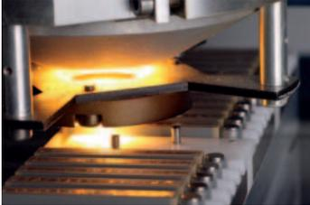
Automated production of PICMA® multilayer piezo actuators in large quantities
