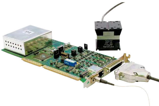
F-206.NCU Rapid NanoAlign Upgrade consists of the P-611 NanoCube® piezo nanopositioner and the E-760 controller card
