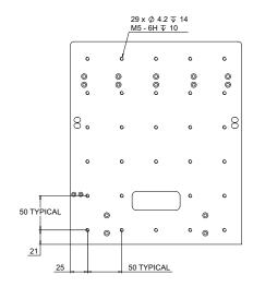
X-AXIS CARRIAGE FRONT PLATE PAYLOAD MOUNTING HOLES
