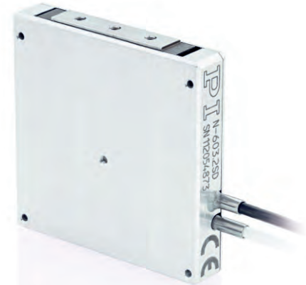
Only 7.5 mm wide and entirely nonmagnetic: The N-603 combines a NEXACT® stepping drive with titanium flexure guides and strain gauge sensor
