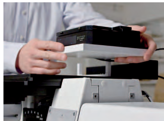
The fine adjustment of the sample is performed by the piezo system that has been integrated in the laser lithography system by Nanoscribe. (Photo: Nanoscribe)
