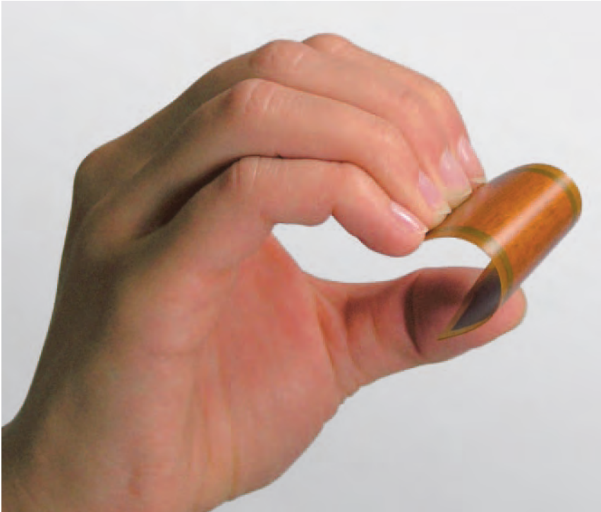
Especially thin piezo ceramics permit bending radii of less than 10 mm
