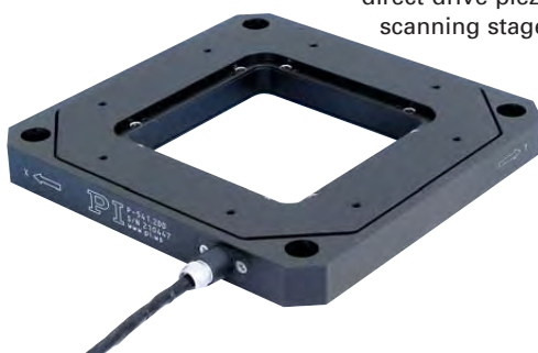
P-541.2DD low-profile, direct-drive piezo scanning stage.
