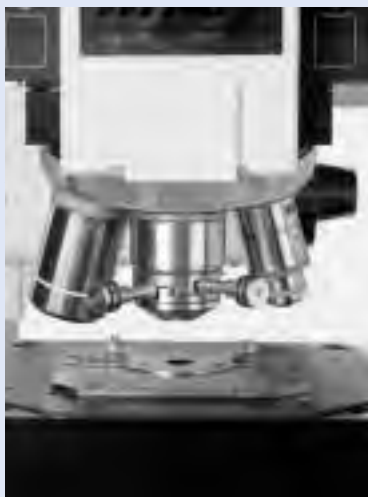
Turret and objectives of a WITec atomic force microscope with P-527 NanoPositioner.
