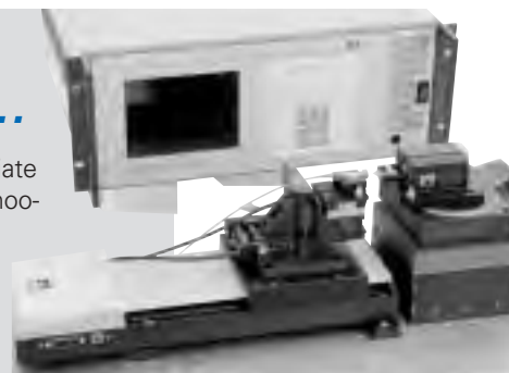
Configuration example from the field of fiber optics: A C-880 controls a combination of (on the left, from bottom to top) M-521.DD (translation stage with 250 mm scanning range in X), 2x M-111.1DG (small translation stages with 5 mm scanning range in Y and Z), Nanocube P-611 (piezo NanoPositioning stage 100 µm in X,Y and Z) and (on the right) M-501.1PD (vertical stage with 12.5 mm travel range in Z), an M-061.DG (rotary stage) and a fiber rotator F-210.DG1 (rotation about the X-axis)
