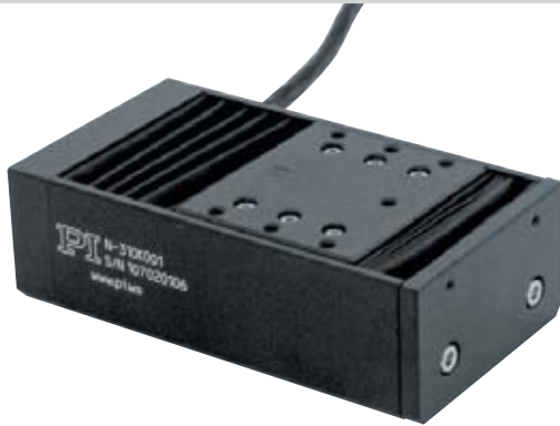
Translation stage with N-310 NEXACT® drive. The positioner offers 20 mm travel range with an encoder resolution of 25 nm
