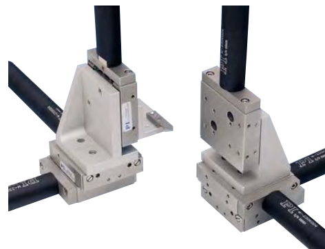
M-231 mounted on M-105 XYZ positioning systems
