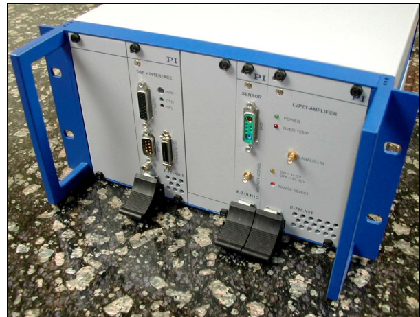
Figure 1. E-712 incorporates a high-power amplifier, a DSP-based servo CPU, 7 th -order sensor conditioning, a patent-pending fast/precise parallel interface with up to 2μsec/command positioning throughput, and feedforward capability for integration into external tracking servos.
