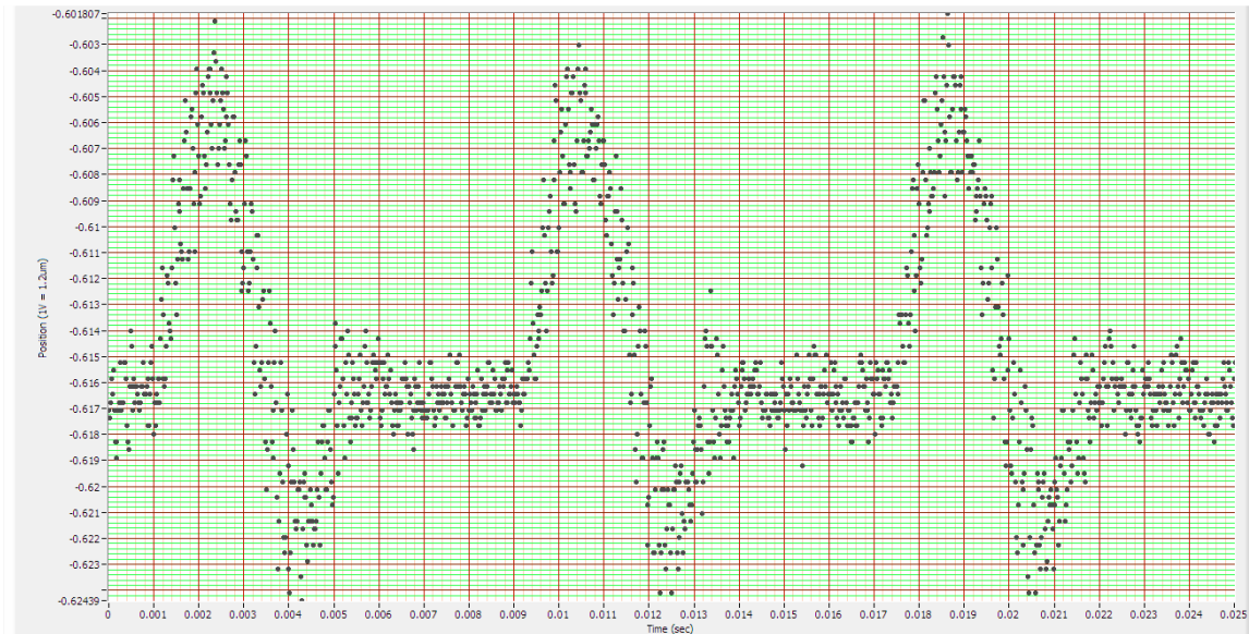
Figure 5. Simulated fast tracking sinusoid, amplitude 25nm; example shown is typical of runout compensation of a disk at 15,000 RPM under control of a track-following servo. During track profiling, nanometer-precise closed-loop increments (flat-line steps) are interleaved between the tool's sinusoidal tracking-and-data-acquisition operations; step-and-settle of these increments are complete within one revolution.
