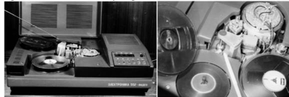
**Fig. 12** Example of the "Elektronika 552-Video" a factory-built video recorder with an ultrasonic motor to power the drive axis, 1982
