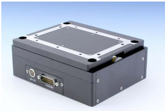
Fig. 11: Hybrid stage for 2nm resolution and 100N load
