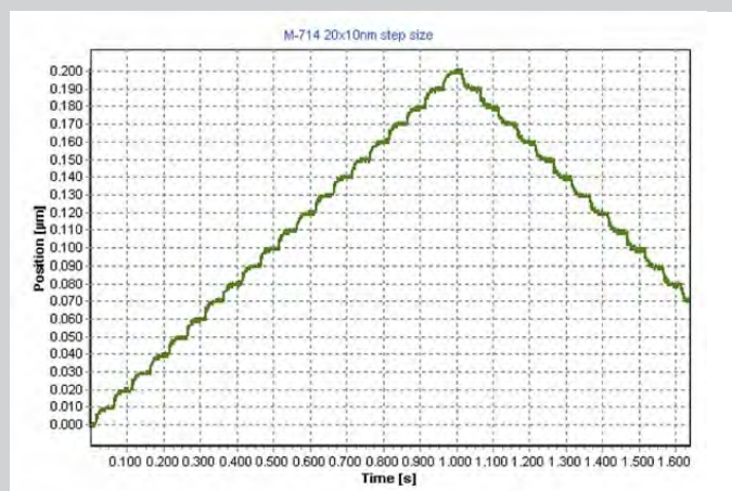
10 nm steps of an M-714 stage, as measured by an interferometer
