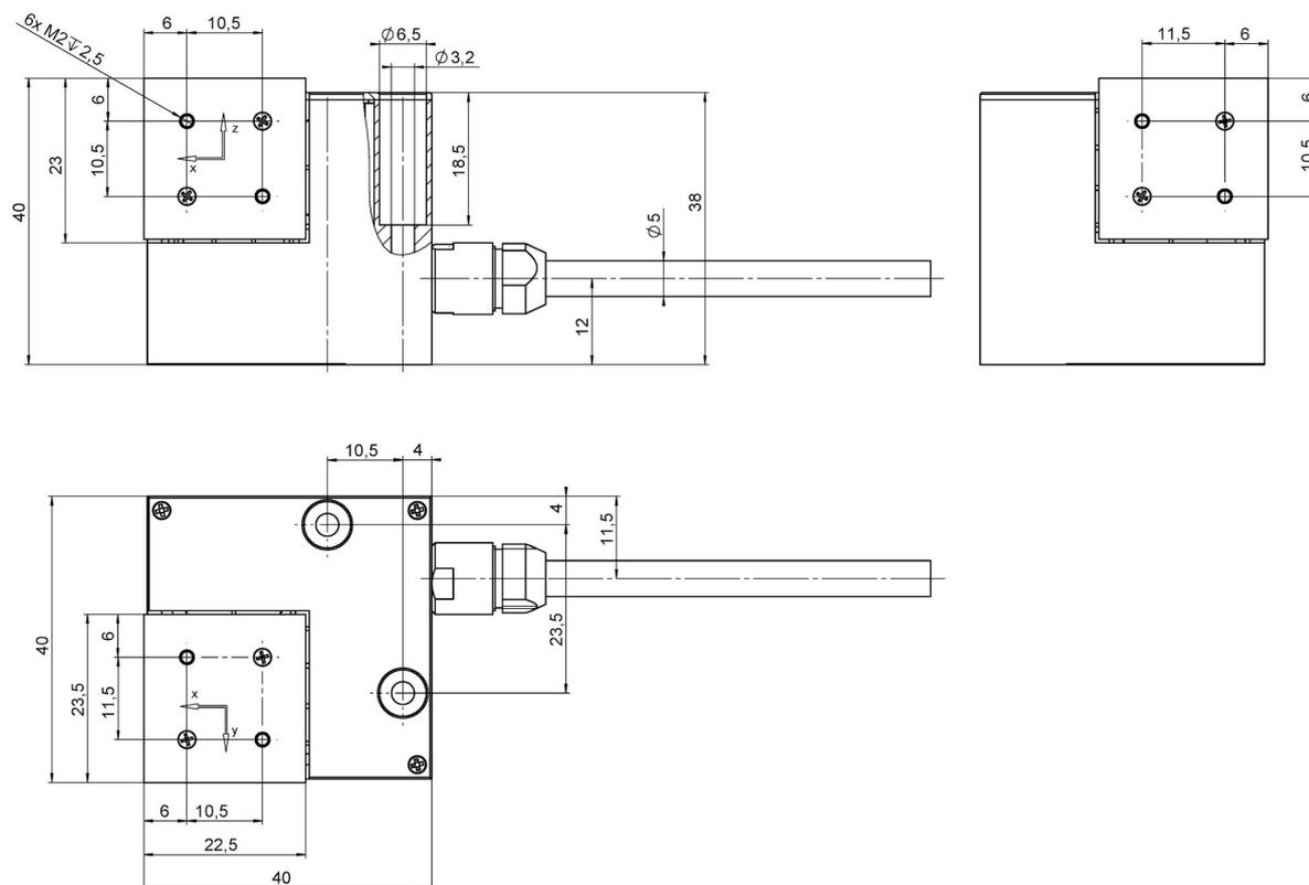
*P-616, Dimensions in mm. Note that the decimal places are separated by a comma in the drawings.*
