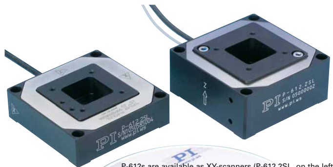
P-612s are available as XY-scanners (P-612.2SL, on the left) and vertical stages (P-612.ZSL, on the right) providing a travel range of 100 \mu\text{m} per axis
