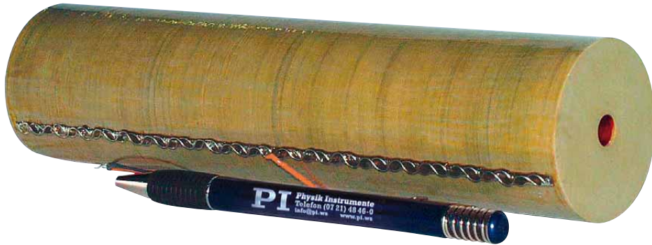
Custom PICA™ Thru piezo actuator with 56 mm outside diameter, 8 mm inner diameter, 250 \mu m displacement. Pen for size comparison
