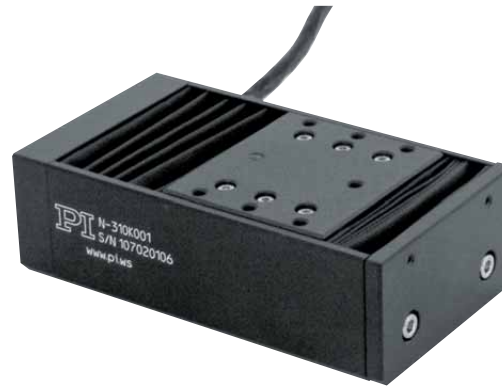
Translation stage with N-310 NEXACT® drive. The positioner offers 20 mm travel range with an encoder resolution of 25 nm
