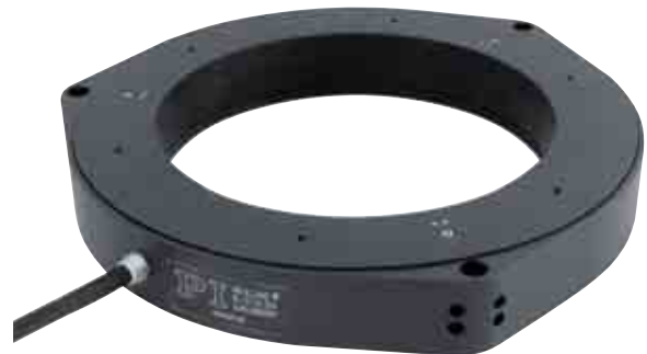
Z / tip / tilt platform with NEXLINE® drives and position sensors; 300 mm (12") diameter, 200 N load capacity, 1.3 mm travel range, 10 mrad tilt range
