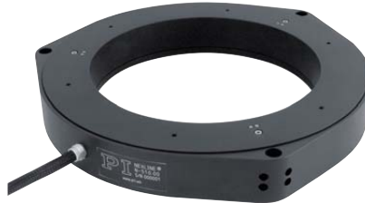
Z, Tip, Tilt platform with NEXLINE® drives and position sensors: 300 mm (12") diameter, 200 N load capacity, 1.3 mm travel range, 10 mrad tilting angle.
