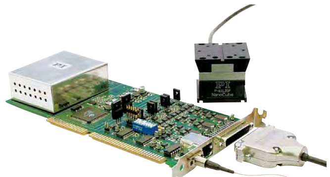
F-206.NCU Rapid NanoAlign Upgrade consists of the P-611 NanoCube® piezo nanopositioner and the E-760 controller card
