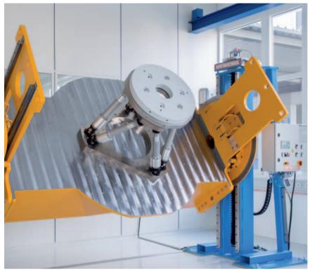
Swivel unit, capable of carrying loads to 7 t, for measurements in application situation
