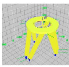
The simulation software graphically displays the position and the available work space of the Hexapod model
