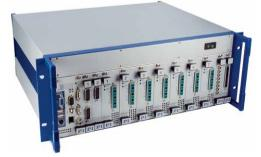
Highly advanced digital controllers are also available for Hexapods with piezo stepping drives which are suitable for operation in strong magnetic fields or UHV environments
