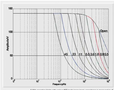
E-504: operating limits with various PZT loads (open-loop), capacitance is measured in  $\mu\text{F}$
