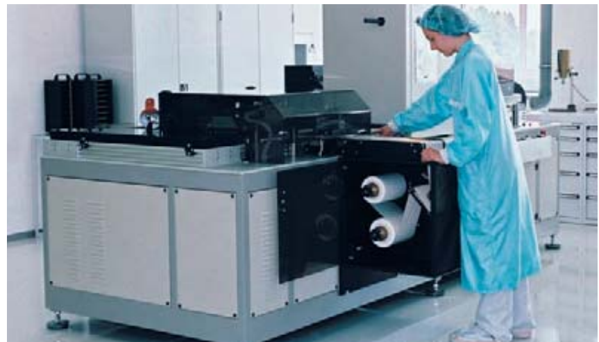
Equipment for fully automated screen printing of electrodes on piezoelectric and dielectric ceramics.
