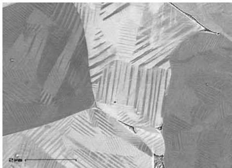
Fig. 2: A cross-sectional view of a ferroelectric ceramic clearly shows the differently polarized domains within the individual crystallites (Source: Fraunhofer Institute for Ceramic Technologies and Systems IKTS, Dresden, Germany)
