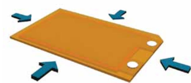
When a voltage is applied, the DuraAct patch transducer contracts laterally
