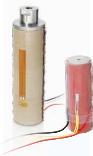
Completely assembled stack actuators with a metal endpiece and SGS expansion sensor (left), with stranded wires, temperature sensor and transparent FEP shrink tubing (right)
