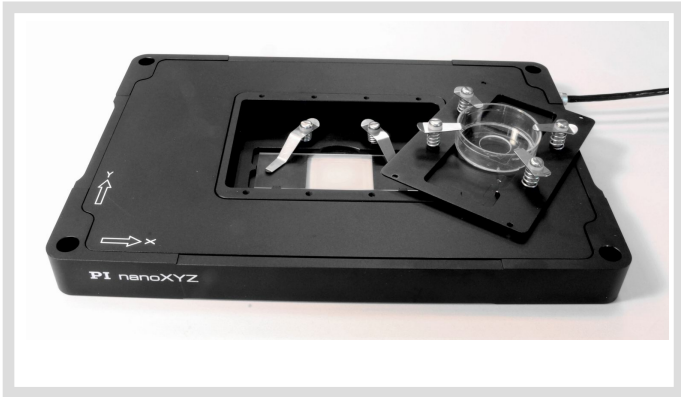
PI nano™ series nanopositioning stages feature a very low profile of 20 mm (0.8"), a large aperture for 1x3" slides and deliver highly accurate motion with sub-nanometer resolution in up to 3 axes. Slide / petri dish holders optional.
