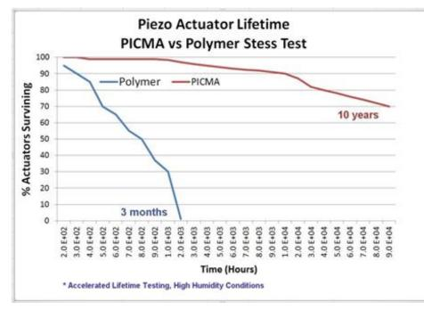
The latest generation multilayer piezo actuators are based on allceramic designs. They can handle high humidity environments, unlike their conventionally polymer insulated siblings.
