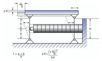
*Piezo flexure actuator with a simple parallelogram flexure guiding system and motion amplifier. The amplification r (transmission ratio) is given by (a+b)/a.*
