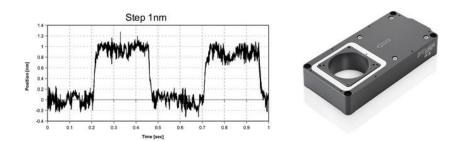
Precision is one of the reasons to chose a piezo flexure guided positioning system. The graph above shows crisp, repeatable subnanometer step response of a <u>P-630 miniature flexure-guided</u> <u>nanopositioning stage</u>, measured with Zygo laser interferometer.
