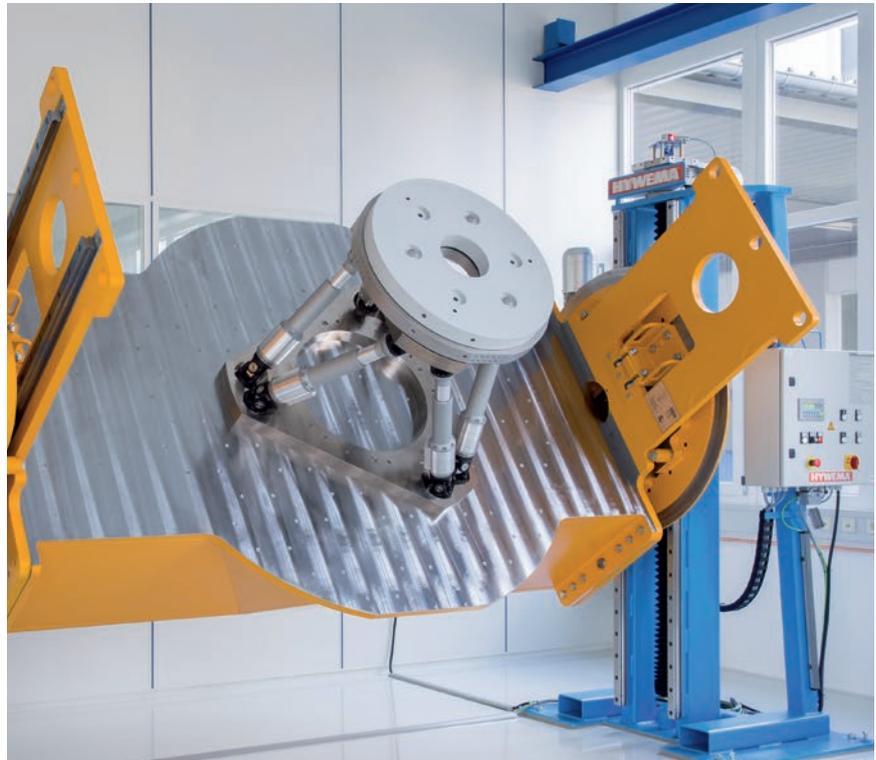
Swivel unit, capable of carrying loads to 7 t, for measurements in application situation
