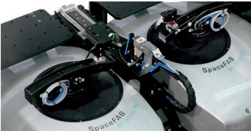
Alignment of optical fibers on a microchip in 6 axes
