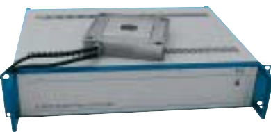
E-710.6CD 6-axis digital piezo controller shown with custom Super Invar 6-DOF piezo flexure NanoPositioning stage (110 V, 25 W, 3 to 6 Channels). See PI Catalog.
