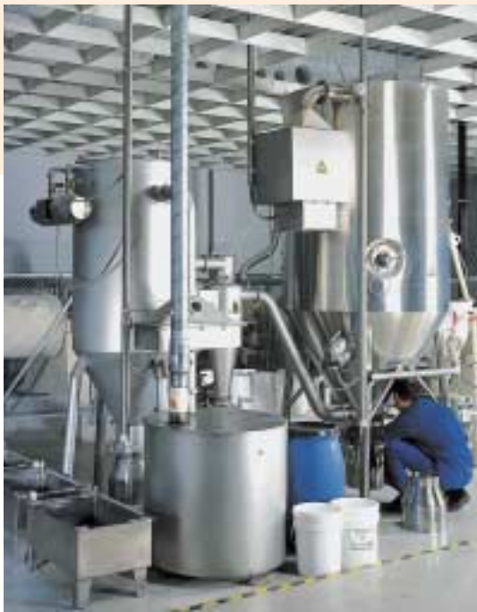
State-of-the-art ceramic spray dryer ensures the highest piezoceramics quality.
