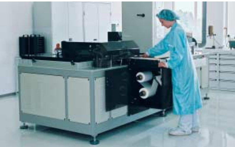
Equipment for fully automated screen printing of electrodes on piezoelectric and dielectric ceramics.
