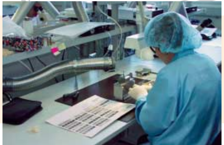
Mounting custom actuator subassemblies for a semiconductor application.
