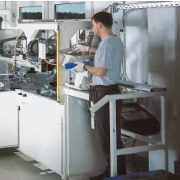
Equipment for fully automated screen printing of electrodes on piezoelectric and dielectric ceramics.
