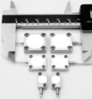
Fig. 16. Two-plate capacitive position sensors provide up to 10,000 times higher resolution than calipers
