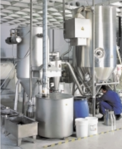
Ceramic spray dryer at PI Ceramic ensures piezo ceramics quality.
