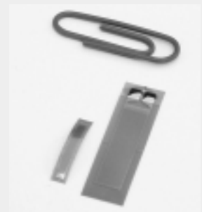
Fig. 13. Strain gauge sensors. Paper clip for size comparison
