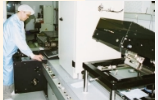
Equipment for multilayer piezo actuator production, at the PI Ceramic factory.
