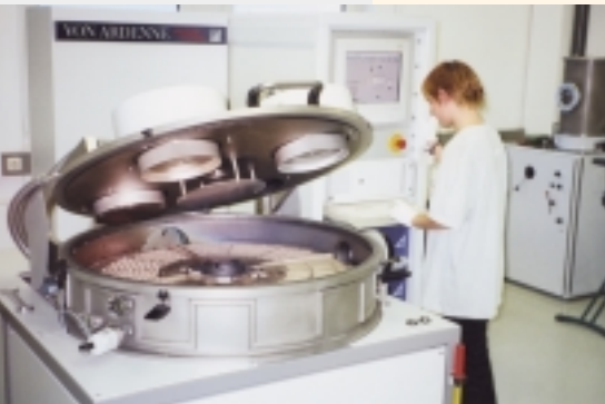
Sputtering (vacuum plating) process of piezo ceramic discs at PI Ceramic.
