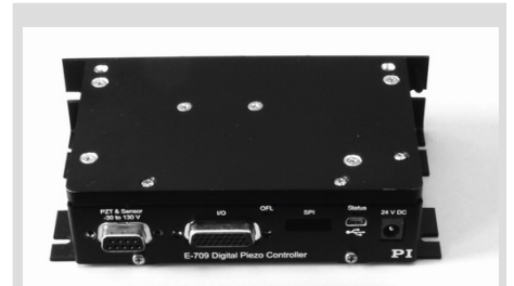
A compact 24 bit piezo controller with USB, RS-232 and a high-bandwidth analog interface is included
