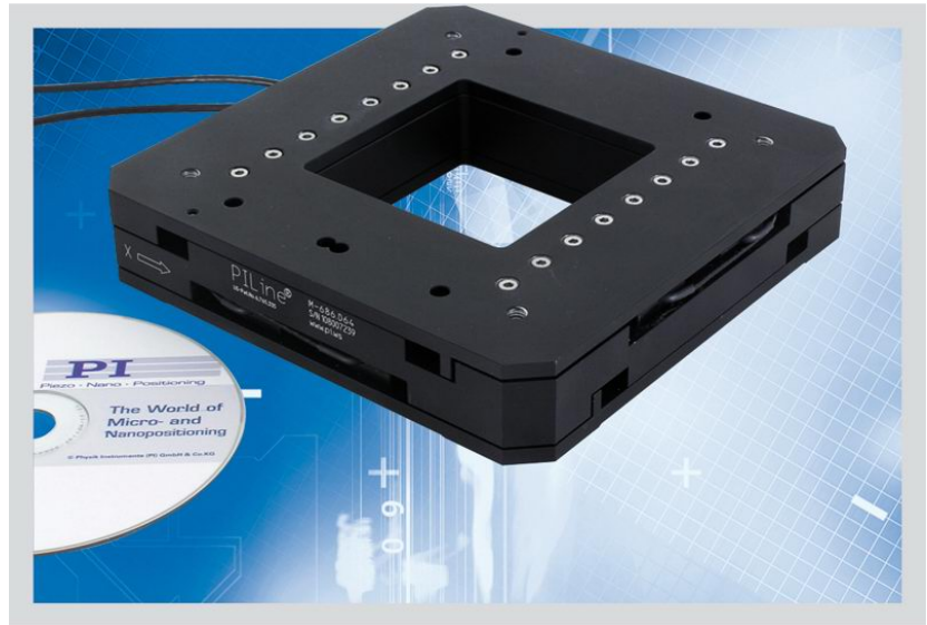
Figure 9. By eliminating the leadscrew assembly, piezomotor long-travel stages provide mm-scale positioning with 0.1\mu\text{m} resolution and nanoscale long-term stability.
