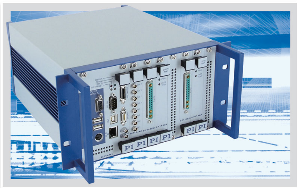
Figure 11. PI's E-712 controller represents the leading edge of nanopositioning controls targeted for SMB applications. With servo update rates to 50kHz and interface options including USB, RS-232, Ethernet, PIO, TTL, analog, and soon SPI, it is ready to enable the next generation of biophysics exploration.
