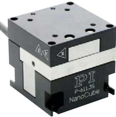
NanoCube® XYZ-nanopositioning system, 100 x 100 x 100 µm closed-loop travel range, resolution 1 nm
