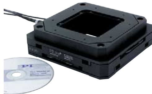
M-686 open-frame stage with P-541.2DD piezo scanner on top, providing a resolution of 0.1 nm and a scanning range of 30 x 30 \mu\text{m} . The system height of the combination with the P-541 XY (or Z) piezo scanner is only 48 mm
