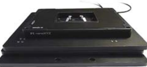
PInano™ XYZ piezo scanner mounted on a M-545.2U Microscope stage. The XYZ piezo nanopositioning stage provides <1 nm resolution and 200x200x200μm scanning range. The high stability and autolocking feature of M-545 provides significant advantages over other microscope stage designs when using fast piezo scanning stages.
