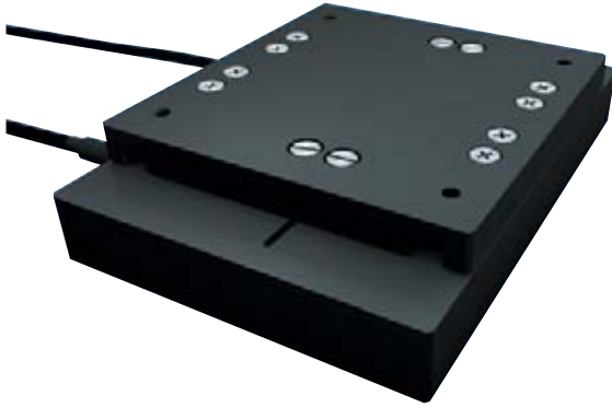
The N-661 miniature linear stage integrates a PiezoWalk® NEXACT® linear motor combined with a high-resolution linear encoder. It provides 20 mm travel and resolution down to the nanometer range.
