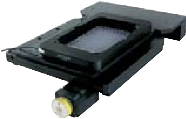
The P-737 piezo Z-stage (shown with multiwell plate) is compatible with motorized microscope XY stages like the one shown from Märzhäuser
