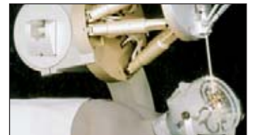
Custom Hexapod designed for neurosurgery Photo: IPA
