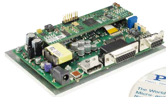
E-709 OEM version board (picture shows version for strain gauge sensors)
