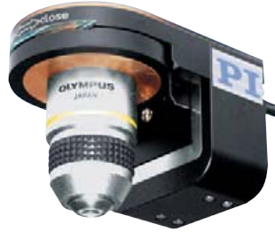
Instead of moving the sample, it is also possible to move the objective. The P-725 PIFOC® Objective Scanner offers travel ranges over 400 µm with nanometer resolution and response times in the millisecond range
