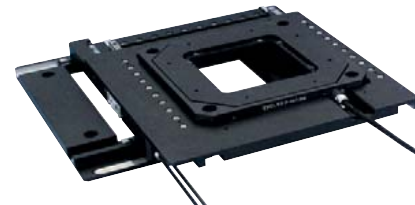
Customized M-686 stage with a bigger footprint, to sink the piezo Z scanner. The system height together with the P-541 piezo scanner is reduced to only 33 mm
