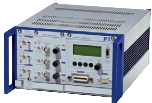
The E-509.E3 servo-controller module in an E-501 9.5" chassis with E-503 piezo amplifier module and E-516 PC-interface/display module provides servo-control of piezo nanopositioning systems with external PISeca™ D-510 capacitive 1-plate sensors
