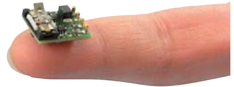
The P-653 miniature drive including the drive electronics measures only 11 mm
