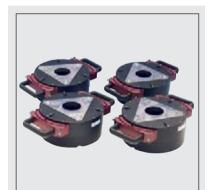
Active tip/tilt mirror system for the Keck Outrigger telescope in Hawaii. The units are controlled by a high-performance digital controller with a fiber optic interface (not shown). Mirror diameter: 250 mm Tip/tilt range: ±150 µrad Resolution: nanoradian range Position measurement: capacitive
