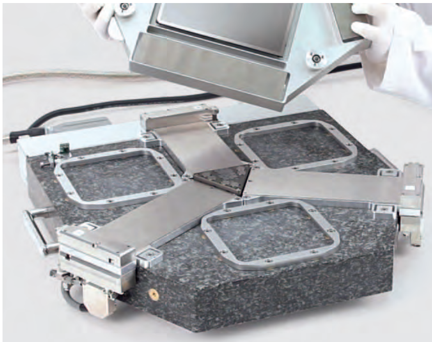
The 6-axis motion is controlled by a 6D sensor. The sensor's reference surface is located in the center below the magnetically levitated platform, a passive component with no need for electrical power or external connection.
