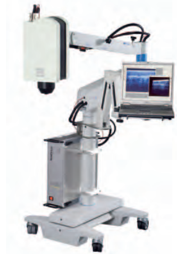
The SkinDex scanner based on OCT technology for non-invasive but reliable examination of the tissue on and under the skin surface (photo ISIS Optronics).
