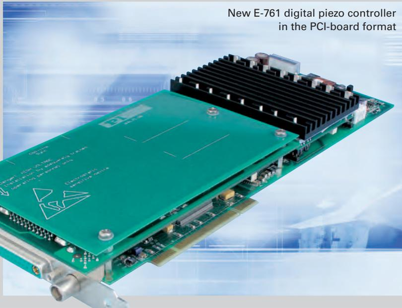
The PCI bus allows for very rapid communication and easy integration with devices such as frame grabbers – a feature which is very advantageous in real-time data acquisition applications or when operating multiple axes or controllers simultaneously.
