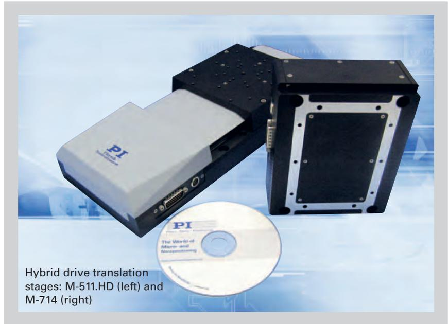
It is the direct integration of PZT actuators into the translation stages and the highly-advanced architecture of the new C-702 hybrid controller that makes it possible to combine piezo-class responsiveness with large travel ranges (up to hundreds of millimeters) and repeatability/resolution of a few nanometers. Compared to high-resolution magnetic linear drives, the hybrid principle also allows high
