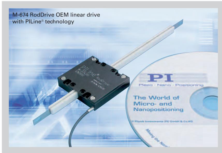
The compact M-674 OEM drives combine high accelerations of over 10 g with top speeds of up to 400 mm/s. Depending on the sensor chosen, loads can be positioned with a resolution of 0.05 µm. PILine® M-674 Rod Drives use ultrasonic piezomotors and are maintenance-free, non-magnetic and vacuum compatible. The travel range, power of the motor and the materials of the linear drives can be flexibly tailored to meet the needs of the customer.
