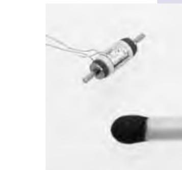
Miniature piezoelectric rotary motor.
