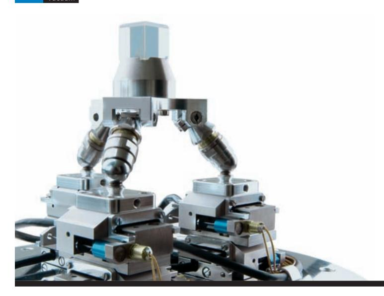
SpaceFAB SF-3000 PS is designed for applications in vacuum environments where probes have to be aligned in all six degrees of freedom. We have minimized the overall dimensions. SpaceFAB SF-3000 PS is based on LPS-30 stages which allow the highest resolution with the piezo inertia drive and a closed loop scale system.
