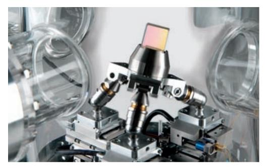
Maximum travel ranges in XY are 12.7 mm with a vertical displacement of only 2 mm; central load of up to 0,5 kg is possible. The pivot point, i.e. the center of the probe, can be set by the customer which is very important for several applications.
