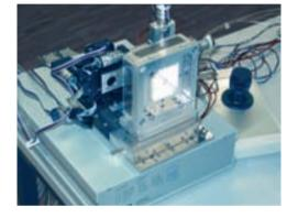
Mini-Positioner MT-55 driven by SMC corvus in a vacuum level of 10<sup>-3</sup> mbar.
